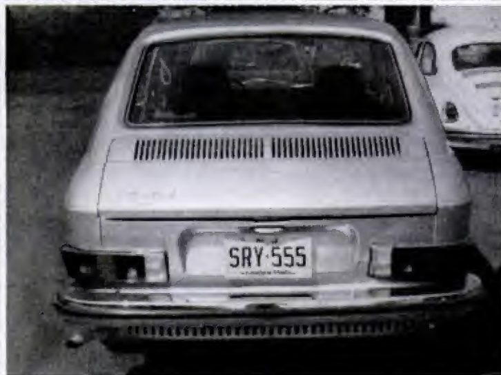
LOUVERS IN LID of the four-door sedan are for the air-cooled rear engine. "Trunk" is in the front
